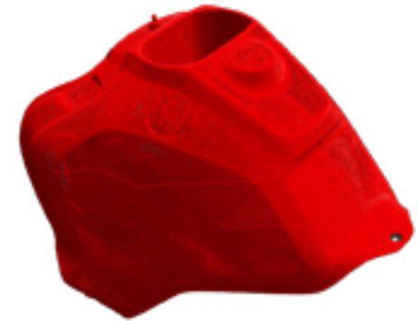
Scanned model of the Carbon Fiber Tank to check geometry.
